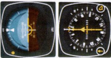
1. The aircraft is flying an OMNI airway in HDG mode on a heading of 080 degrees.
