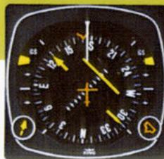
2. Capturing the ILS course can be accomplished without overshooting or bracketing with the same technique you used in intercepting an enroute course. Simply keep the top of the deviation bar on the lubber line and coordinate your turn until the bar is centered with the course arrow. Each dot on the LOC deviation scale represents 1/2 a degree of deviation when tuned to an ILS frequency.
