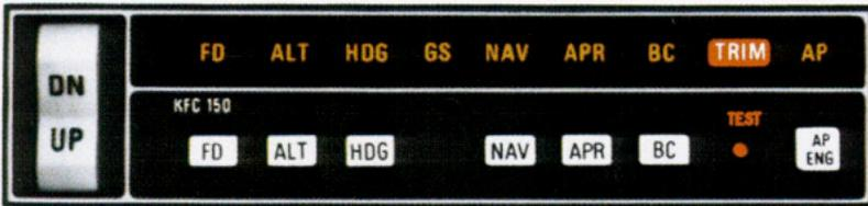
The KAP 150 system incorporates a system self-test function which is activated by a test button on the KC 191 Mode Control/Computer/Annunciator. The test must be performed before the autopilot can be engaged. The test determines, before takeoff, that the system is operating normally. To perform a test — momentarily push the test button:
