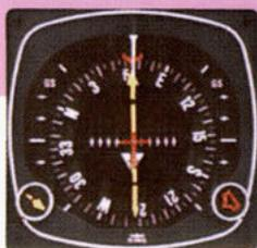
1. Approaching the STL VORTAC, the controller asks you to hold southwest of the VORTAC on the 244 degree radial, right turns. You are now over the station with a 064 degree course selected (the TO/FROM indicator has swung to "FROM"). Set your heading bug to the reciprocal or outbound heading of 244 degrees for easy reference and begin your right turn holding pattern.
