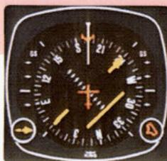
2. During the procedure turn outbound, the deviation bar shows pictorially that the aircraft (as represented by the symbolic aircraft in the center of the KI 525A) is flying away from the localizer centerline at a 45 degree angle when the heading bug is under the lubber line. Note that left-right deviations of the course bar give "fly-to" indicators, just as on the front course.
