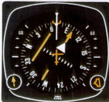
NOTE: You should consider using HDG select mode just prior to VOR station passage. If the autopilot is engaged in NAV mode it may cause erratic maneuvers while following a rapidly changing course deviation needle as the aircraft flies in the cone of confusion.
