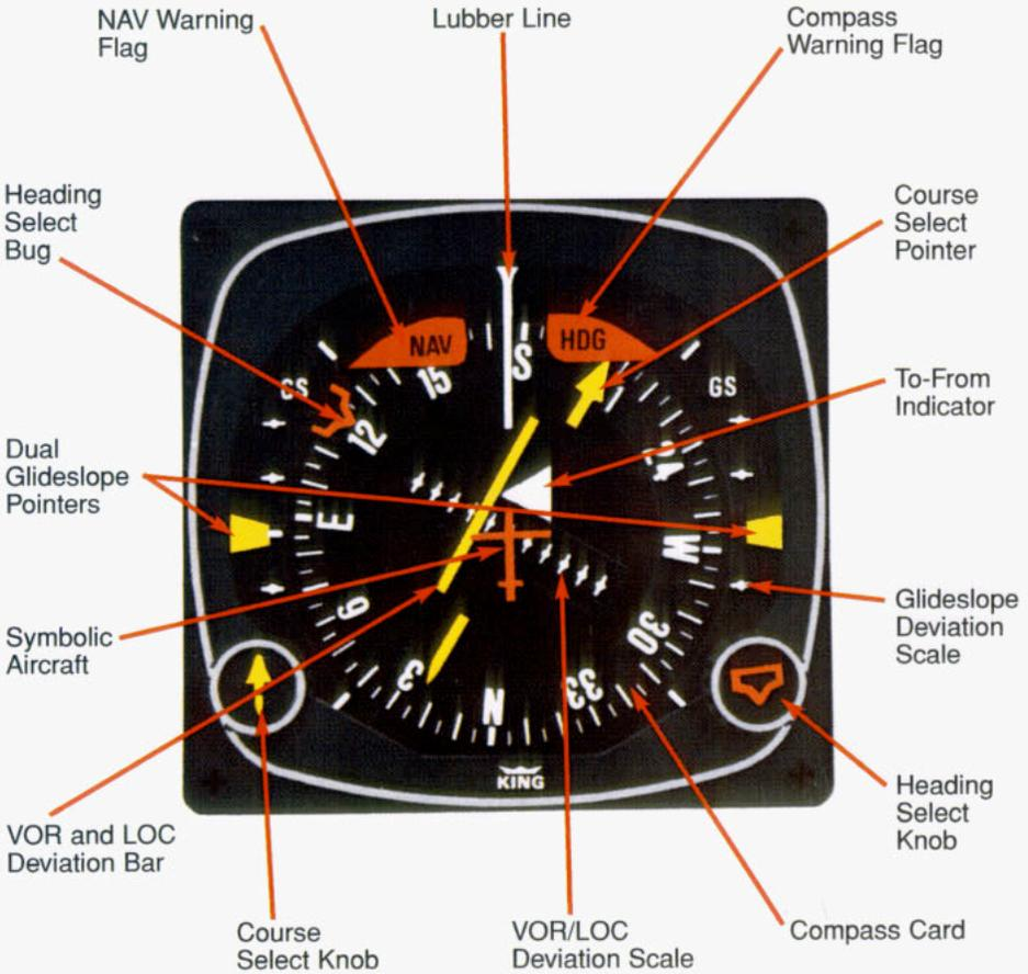
The KI 525A Pictorial Navigation Indicator is the panel display for the KCS 55A Compass System. It replaces the standard Directional Gyro and Course Deviation Indicator (CDI) in the aircraft's panel, combining slaved heading and VOR/LOC/Glideslope deviation information into one compact display. By providing a simple, comprehensive visual presentation of the aircraft's heading and position in relation to a desired course, the pilot's navigation workload is considerably reduced.
