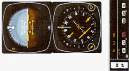
3. During the procedure turn outbound, the deviation bar shows pictorially that the aircraft is flying away from the localizer centerline at a 45 degree angle on a selected heading of 283 degrees.
