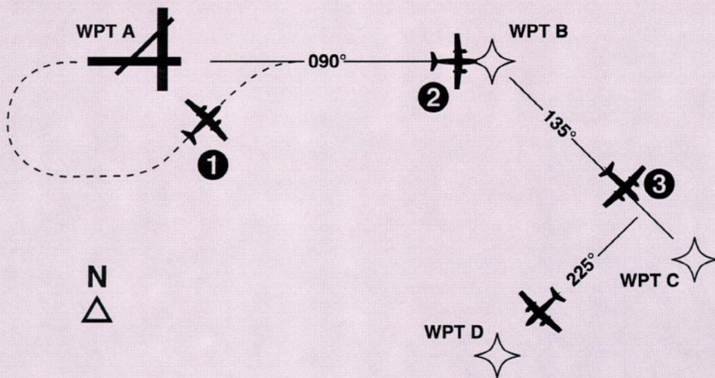
**Objective:** Intercept the desired course and complete a "direct to" operation after passing waypoint "B" while coupled to a Long Range Nav.
