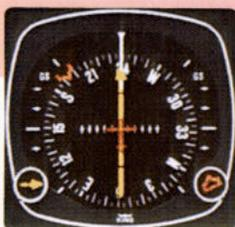
1. You are outbound on the back localizer course, having already set the course pointer to the inbound front course at 238 degrees. The heading bug is preset at 193 degrees for the procedure turn. (Since there is usually no glideslope signal on a back course, the glideslope pointers are out of sight.)
