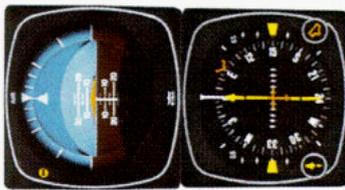
3. The capture sequence starts when NAV mode is automatically engaged canceling the NAV/ARM and HDG modes. The V-bar is calling for a right bank which is being satisfied by the autopilot.
