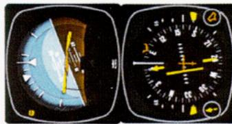
4. The aircraft has completed its turn to the 112 degree course. A wind correction produces an aircraft heading of 105 degrees, displaying a seven degree "crab" angle to maintain the 112 degree course.
