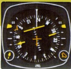
1. You are vectored from the holding pattern to the 13 DME arc. The aircraft is turning, with the heading bug set on 170 degrees to intercept the localizer. You have already set the selected course pointer on the inbound ILS course 130 degrees and the KI 525A shows the localizer course is directly ahead. The glideslope pointers came into view when the ILS frequency was tuned, since a usable glideslope signal is being received.
