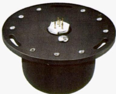
The **KMT 112 Magnetic Slaving Transmitter** senses the direction of the earth's magnetic field and continuously transmits this information through the slaving circuitry to the directional gyro which is automatically corrected for precession or "drift". This sensor is mounted remotely — usually in a wing tip — to eliminate the possibility of magnetic interference.
