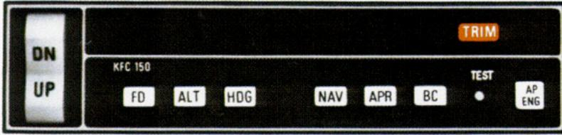
When initially powered (no modes selected), the KFC 150 will display aircraft attitude on the FCI and aircraft heading on the PNI. The V-bar will be biased out of view. The trim light will be lit on the KC 192 as a reminder of the need to perform the system self-test.
