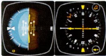
2. A waypoint has been established and the RNAV computer is in enroute mode. A 112 degree course to the waypoint has been selected and "NAV" mode button pushed "on". The "NAV" light is flashing to signify that the NAV mode is armed. The autopilot is still following the heading select mode on 080 degrees and will do so until the capture zone is entered and NAV mode is engaged. The capture point is now being computed based on closure rate.
