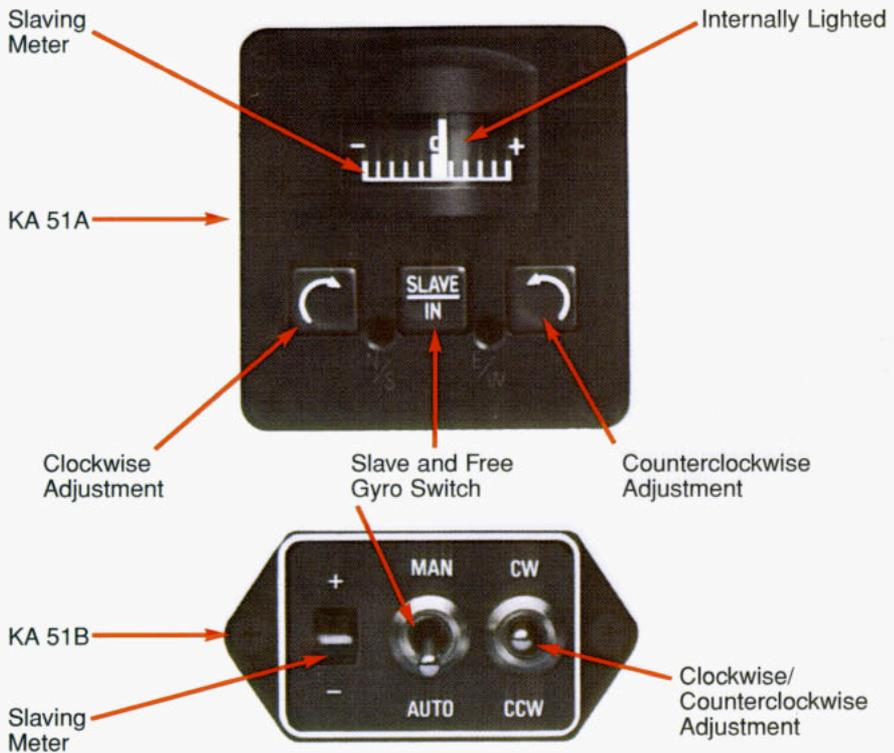
**Slaving Meter** - This meter indicates any difference between the displayed heading and the magnetic heading. Right or up deflection indicates a clockwise error of the compass card. Left or down deflection indicates a counterclockwise error of the compass card. Whenever the aircraft is in a turn and the card rotates, it is normal for this meter to show a full deflection to one side or the other.
