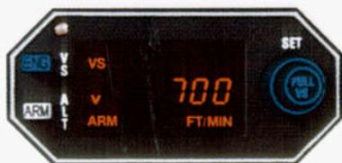
Operation of the autopilot in descent is identical to operation in climb with a pitch round out allowing a smooth capture of the assigned altitude.
