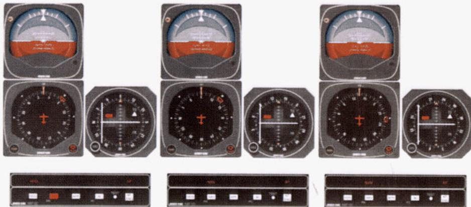
1. The aircraft is engaged in Heading (HDG) and Altitude Hold (ALT) mode. A flight plan from waypoint "A" to "B" to "C" is entered in the Long Range Nav. NAV Arm is activated by pressing the NAV button. The Heading Bug, which acts as the course pointer, is then selected within five seconds to 090°. The autopilot commands a 045° intercept until coupled. Upon coupling, the autopilot tracks the Long Range Nav.
