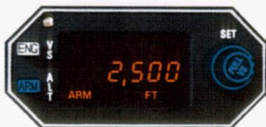
4. In preparation for the descent, the new altitude is preset in the KAS 297B. When the descent is to be started, the new altitude is ARMed, the inner concentric knob is pulled out, the desired vertical speed is entered and the ENG button is pushed with vertical speed displayed.
