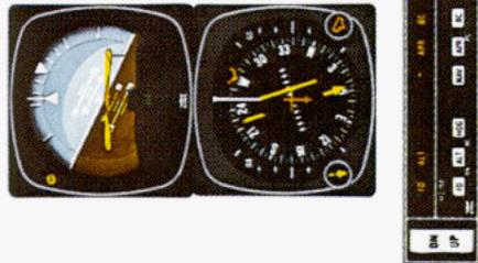
2. When the computed capture point is reached the approach mode is automatically activated and a left turn outbound on the localizer is commanded by the flight director, and is satisfied by the autopilot. Note that the left-right deviations of the bar give "fly-to" indications just as on the front course inbound.
