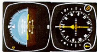
1. The aircraft is flying an OMNI airway in HDG mode on a heading of 080 degrees.
