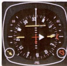
4. Halfway through your turn to the inbound 064 degree course, the KI 525A shows the symbolic aircraft approaching the deviation bar at a right angle. By keeping the top of the deviation bar on the lubber line, you can complete your turn and roll out precisely on course.
