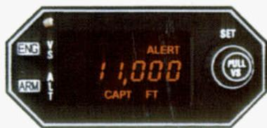
1. You have lifted off having previously set the assigned altitude of 11,000 feet. When a safe altitude is reached, the autopilot is engaged, altitude is ARMed, and the aircraft is climbing to the assigned altitude in pitch attitude hold. Once a stable rate of climb is established, the engage (ENG) button is pushed while the selected altitude is showing; engaging VS at its present value. The KAS 297B will automatically display this vertical speed for 2 seconds after pushing VS ENGage.
