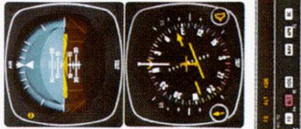
4. Desired altitude has been reached, altitude hold (ALT) has been engaged and the aircraft has returned to level flight. The 010 degree heading has been acquired.
