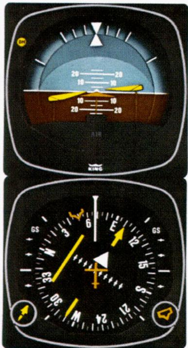
**NOTE:** You should consider using HDG select mode just prior to VOR station passage. If the autopilot is engaged in NAV mode it may cause erratic maneuvers while following a rapidly changing course deviation needle as the aircraft flies in the cone of confusion.
