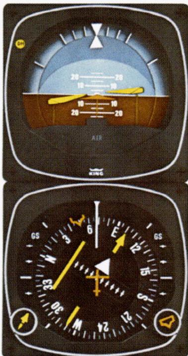
When the intercept occurs, "GS" is illuminated on the annunciator panel. The V-bar commands the pitch necessary to maintain the glideslope. If the autopilot is engaged it will satisfy these commands. If the altitude hold (ALT) mode had been engaged prior to GS capture, it will disengage at capture and the "ALT" light will go out.
