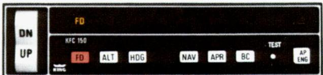
If a change in pitch attitude is desired, the control wheel steering (CWS) button on the pilot's control wheel can be used to synchronize the V-bar (in the FD mode with autopilot disengaged) without removing your hand from the control wheel.
