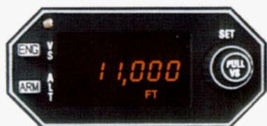
3. You have now reached the assigned altitude of 11,000 feet and the autopilot has automatically engaged altitude hold.
