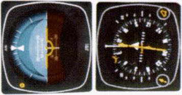
4. The aircraft has completed its turn to the 112 degree course. A wind correction produces an aircraft heading of 105 degrees, displaying a seven degree "crab" angle to maintain the 112 degree RNAV course.
