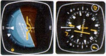
3. The capture sequence starts when NAV mode is automatically engaged canceling the NAV/ARM and HDG modes. The autopilot is turning the aircraft right.
