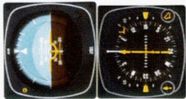
2. The autopilot is following the localizer. At the outer marker, the glideslope deviation needle is at midscale. Altitude hold is automatically disengaged when the glideslope is captured. The "ALT" light goes out and "GS" comes on. The autopilot will make pitch and bank changes as necessary to maintain localizer and glidepath.
