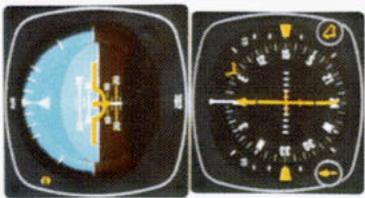
3. At the middle marker, the autopilot is disconnected with the button on the control wheel. This cancels all operating autopilot modes. The pilot initiates a missed approach.
