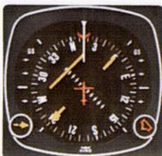
3. Now you've reset the heading bug to 013 degrees and made a 180 degree turn to this heading. This 013 degree heading will intercept the back course. The KI 525A clearly pictures the course you are to intercept and the angle of interception.
