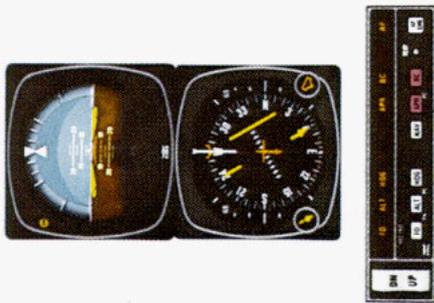
1. In heading select (HDG) and altitude hold (ALT) mode, the aircraft is heading 270 degrees toward the localizer. The front inbound localizer course of 058 degrees is selected. APR mode and BC mode are selected to go outbound on the front course. The capture point is now being computed, based on closure rate. (APR light is flashing to indicate the approach mode is armed.)
