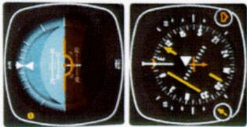
2. A waypoint has been established and the RNAV computer is in enroute mode. A 112 degree course to the waypoint has been selected and "NAV" button pushed "on". The "NAV" light is flashing to signify that the NAV mode is armed. The autopilot is still following the heading select mode on 080 degrees and will do so until the capture zone is entered and NAV mode is engaged. The capture point is now being computed based on closure rate.
