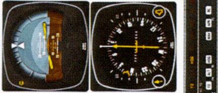
2. The heading "bug" on the PNI is turned to the new desired heading of 010 degrees and the aircraft begins to respond with an immediate left turn just as the autopilot mode is engaged by depressing the "AP" button.
