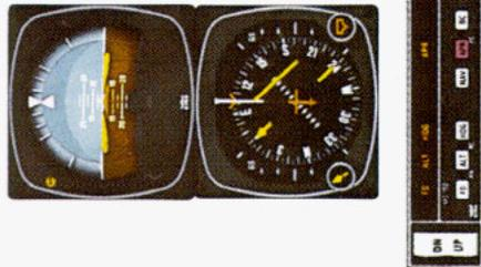
4. Now you have reset the heading "bug" to 103 degrees and made a 180 degree turn to this heading. This 103 degree heading will intercept the front course of 058 degrees. You must now reselect the approach mode by depressing the APR button on the mode controller. The APR light will begin to flash signifying the approach mode is armed. The PNI clearly pictures the course you are to intercept and the angle of interception. Automatic capture of the localizer will occur.
