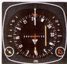
3. Outbound, you are using the heading bug as a reference for 244 degrees. The 244 degree radial is off the right wing and parallel to your outbound course.
