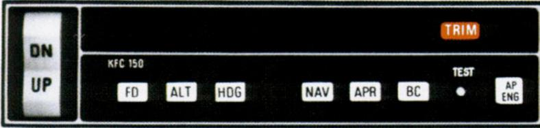
When initially powered (no modes selected), the KAP 150 will display aircraft attitude on the KG 258 and unslaved heading on the KG 107. Align heading to the magnetic compass by pushing and rotating the knob on the lower left of the KG 107 and update periodically to correct for preces-
