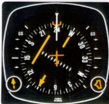
5. The autopilot will fly the selected heading until entering the capture zone, then turn to intercept the course. The "HDG" light will go off and the "APR" light will illuminate steadily as the BC mode goes from arm to engage.
