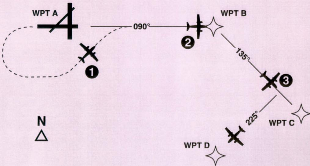
**Objective:** Intercept the desired course and complete a "direct to" operation after passing waypoint "B" while coupled to a Long Range Nav.
