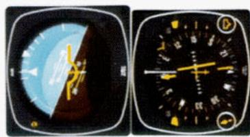
1. Continuing the maneuver on page 52, APR coupling course ("APR" light comes on steady, "HDG" light goes off), and the glideslope mode is automatically armed. The autopilot will roll the aircraft out on localizer and the course index will center.
