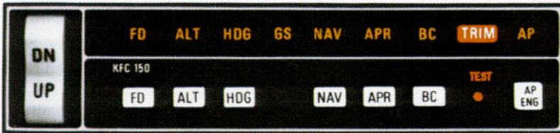
The KFC 150 system incorporates a system self-test function which is activated by a test button on the KC 192 Mode Controller/Computer/Annunciator. The test must be performed before the autopilot portion of the system can be used, but need not be performed before using the flight director portion. This test determines, before takeoff, that the system is operating normally. To perform a test — momentarily push the test button. The following actions will occur:
