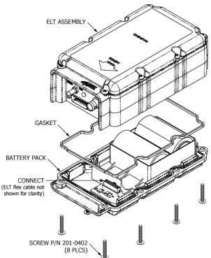
Figure 28 Battery Pack Installation
