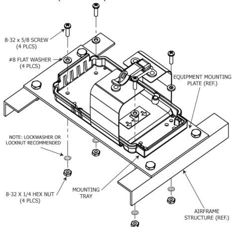
**Figure 14 Typical Mounting Tray Installation**
