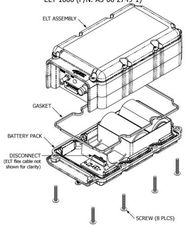
**Figure 11 Battery Pack Removal**
