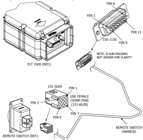
**Figure 24 Remote Switch Harness Arrangement**
