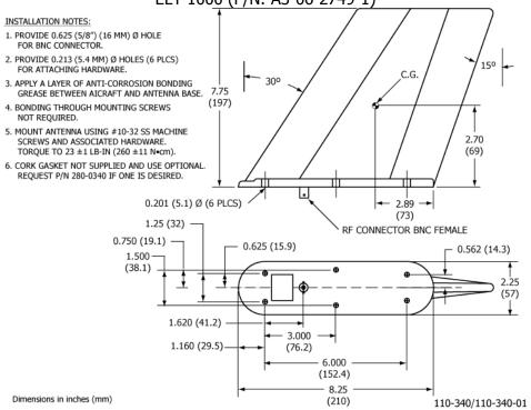
Figure 16 Blade Antenna 110-340 Outlines and Dimensions
