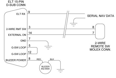
Figure 20 Typical 2-Wire Installation for Unshielded Harness
