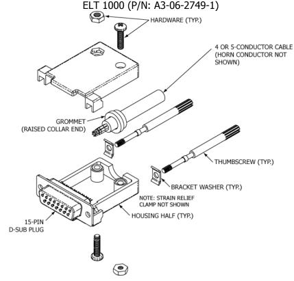
**Figure 25 Harness Plug Assembly**
