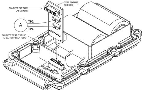
**Figure 7 Current Draw Test Setup**
