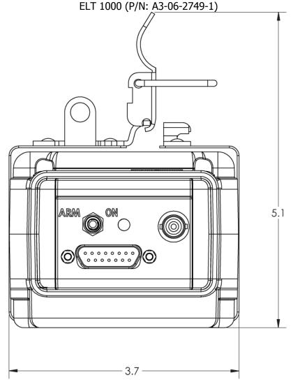
Figure 13 ELT 1000 Metal Strap Minimum Clearance Dimensions
