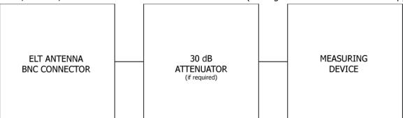
**Figure 6 Performance Test Setup**
