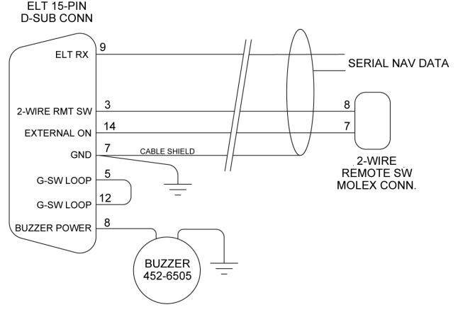
Figure 21 Typical 2-Wire Installation for Shielded Harness
