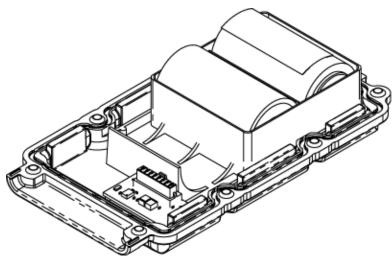
**Figure 4 Battery Pack Assembly**
