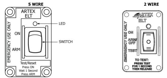
**Figure 2 Remote Switch Front View**
