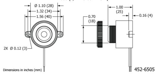
**Figure 19 Buzzer Outline and Dimensions**
