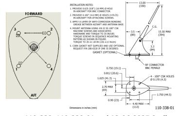
Figure 15 Rod Antenna 110-338, 110-338-01 and A3-06-2835 Outlines and Dimensions
