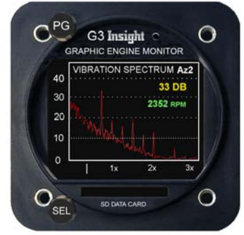
4 - Engine Vibration Screen
