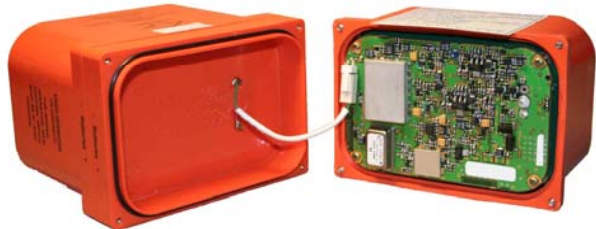
Figure 16: Battery Replacement for ELT Main Unit (Actual View).
