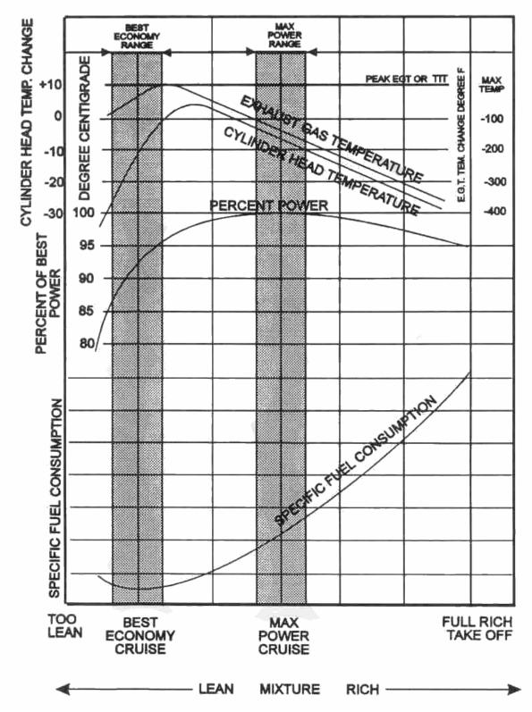
THIS REPRESENTATIVE DIAGRAM SHOWS THE EFFECT OF LEANING ON: CYLINDER HEAD TEMPERATURE, EXHAUST GAS TEMPERATURE OR TIT, ENGINE POWER, AND SPECIFIC FUEL CONSUMPTION FOR A CONSTANT ENGINE RPM AND MANIFOLD PRESSURE.
