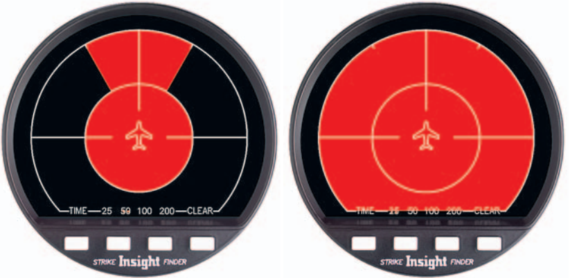
Figure 17. CAUTION and DANGER Areas
